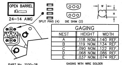
THE OPEN BARREL CRIMP DIE HAS TO BE PINNED IN PLACE FOR PROPER OPERATION USING THE FOUR SPLIT PINS PROVIDED.
