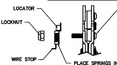
REPLACE LOWER JAW SCREW WITH LONGER SCREW. TIGHTEN UP SCREW, MOUNT LOCATOR AS SHOWN, ATTACH USING LOCKNUT. LOOSEN ASEMBLY TO MAKE SURE WIRE STOP MOVES FREELY.
