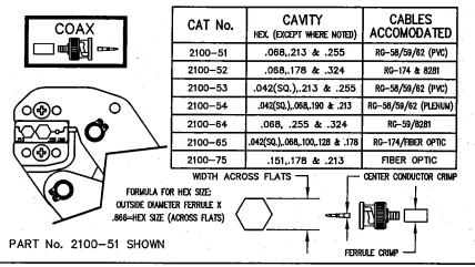
Strip cable according to manufacturer's specifications. Select proper hex cavity for size of cable being used. Crimp center conductor in area shown. Assemble connector and crimp outer ferrule.
